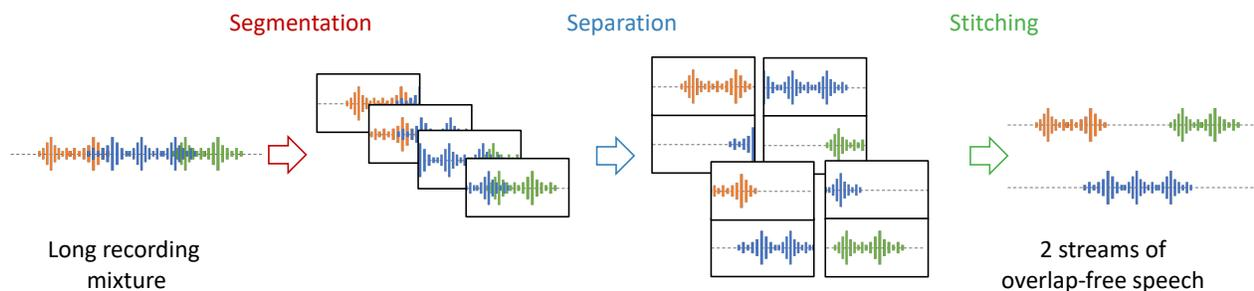
**Fig. 1.** A typical pipeline for continuous speech separation systems. The *segmentation* step splits the long recording into short blocks. The *separation* step performs separation on the blocks. The *stitching* step concatenates the block-level separation outputs to long streams which only contains nonoverlapped targets.
