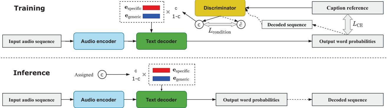
**Fig. 1.** Proposed neural conditional captioning framework. During **training**, the text decoder takes the reference condition and the encoded audio embedding as the input to give word probabilities. During **inference**, we manually assign the condition and feed to the text decoder to control the output set-diversity.
